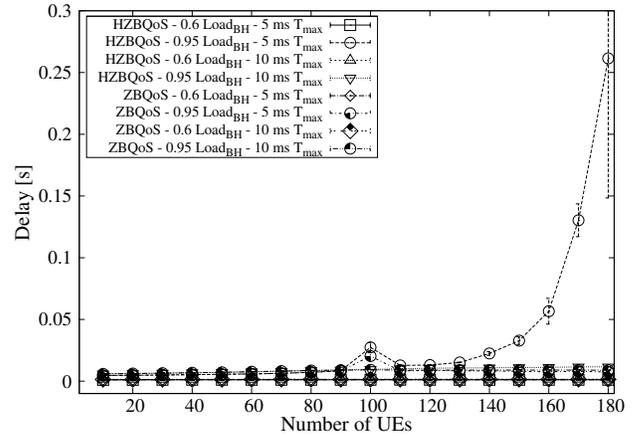
Figure 8. Average Packet Delay in the Backhaul for Video Traffic
