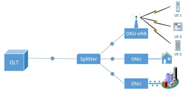
Figure 1. LTE/TDM-PON Integrated Network Architecture
