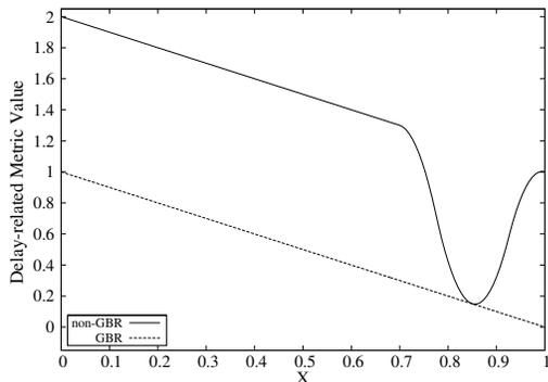
Figure 2. Delay-related metric value for GBR and nGBR bearers as a function of the ratio  $x$
