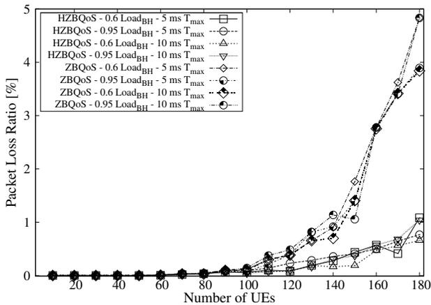
Figure 3. Packet Loss Ratio for Video Traffic
