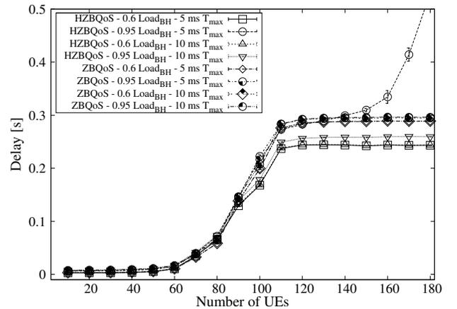
Figure 5. Average Packet Delay for CBR Traffic
